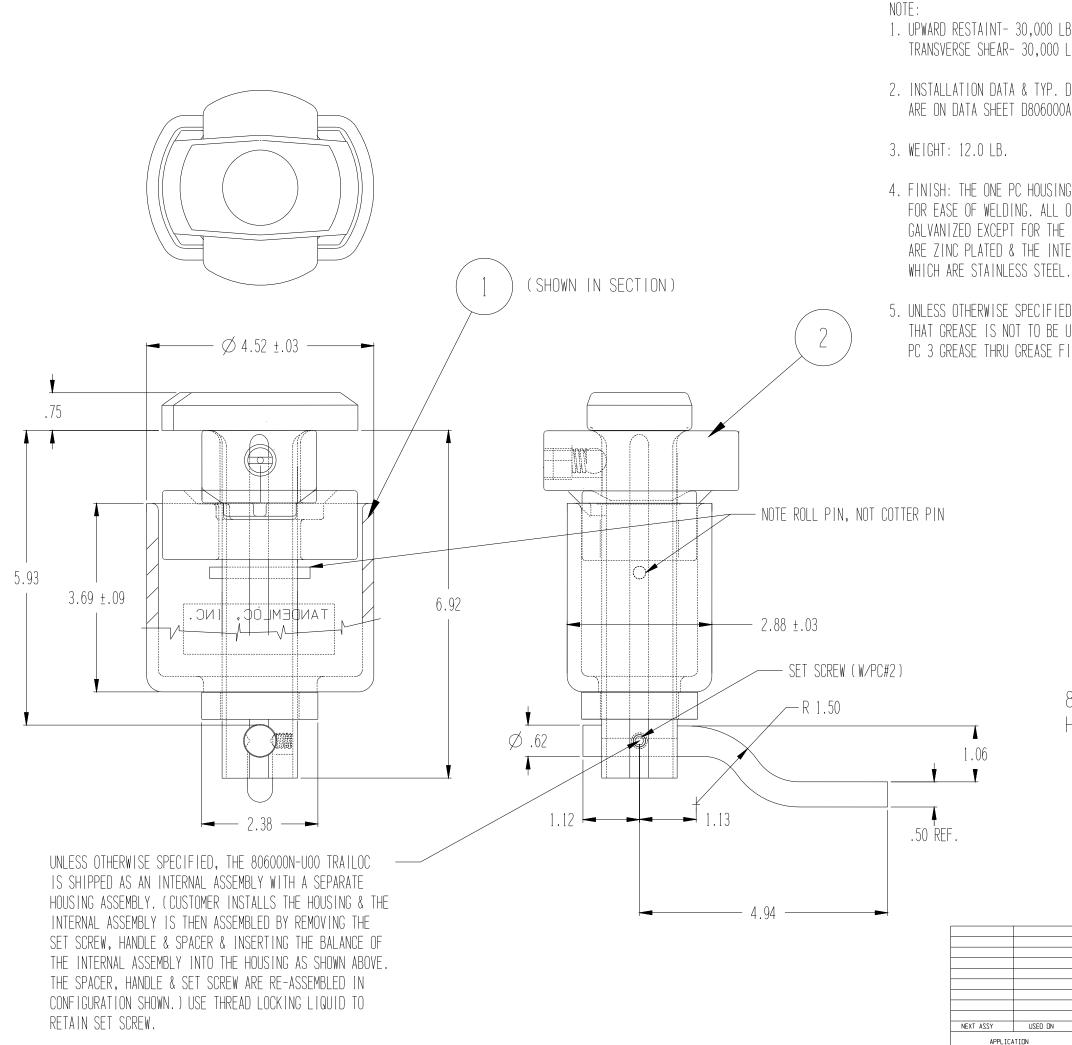
1. UPWARD RESTAINT- 30,000 LB. ULT. TRANSVERSE SHEAR- 30,000 LB.
